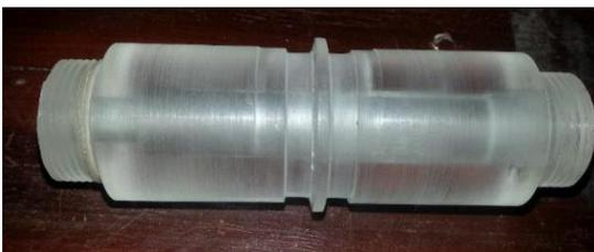
Gambar 10. Body Probe Bobbin Differential
