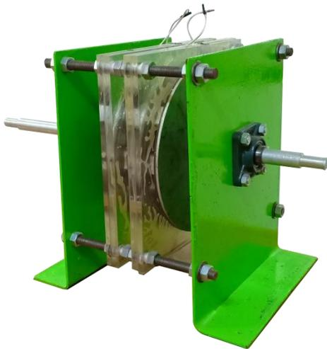
Gambar 3. Hasil rakitan purwarupa generator magnet permanen fluks aksial *multistage*
