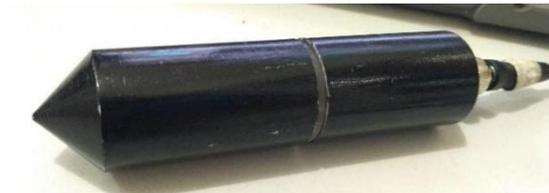
Gambar 11. Probe Bobbin Differential
